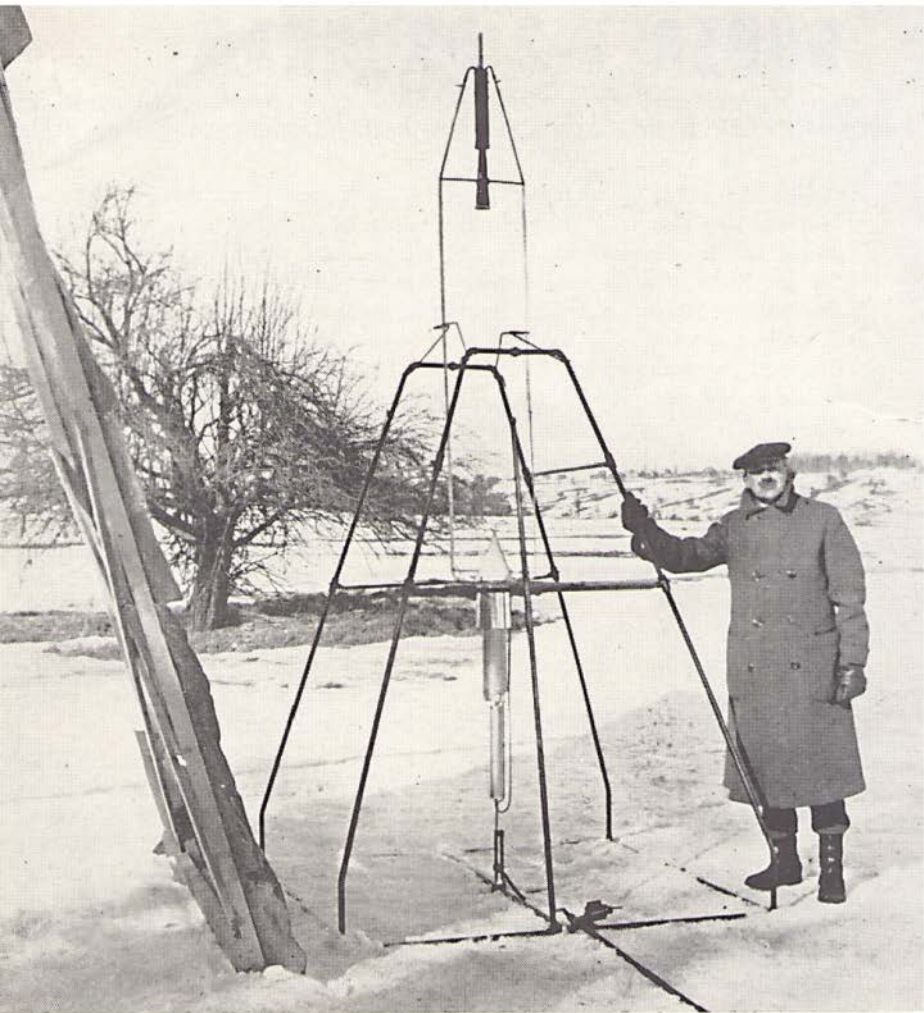
Dr. Robert H. Goddard stands by his first successful liquid propellant rocket on the Ward Farm, Auburn, Massachusetts. The date: March 16, 1926. Rocket propellants used: liquid oxygen and hydrocarbon (gasoline).
